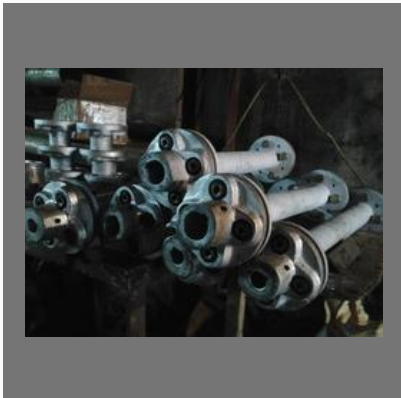
Drive Shaft For Cooling Tower
