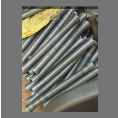
Pvc pipe bending spring
