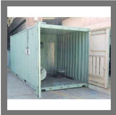
Shot Blast Room
