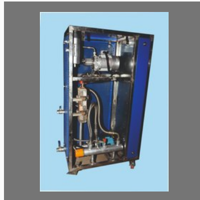
Fuel Conditioning Unit
