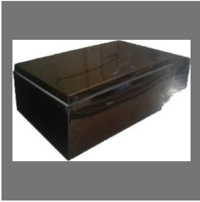
Water bath for temperature thermoplastic sheet
