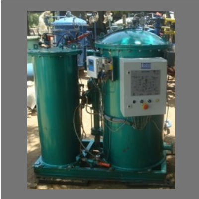
Oily Water Seperator
