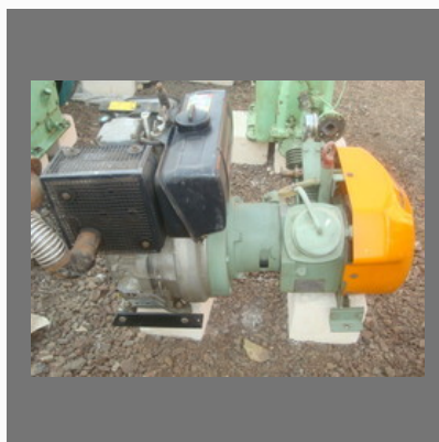
Emergency Air Compressor
