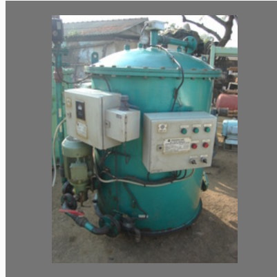
Oily Water Seperator
