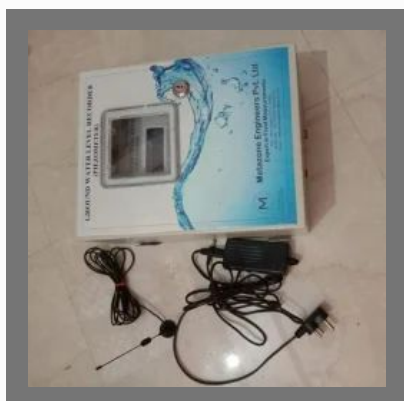
Ground Water Level Recorder Piezometer
