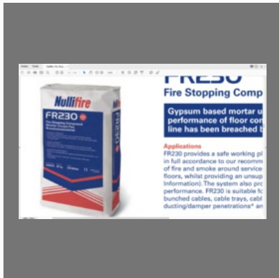
FR230 Fire Stopping Compound Gypsum based mortar used to reinstate the fire resistance performance
