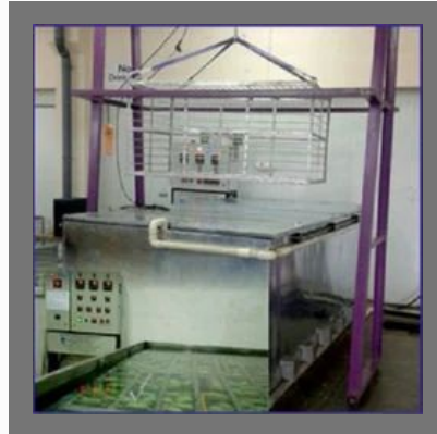
Hot Water Treatment Plant For Mangoes Export
