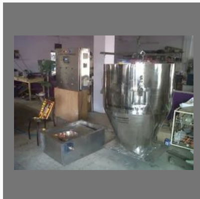
Automatic Weighing and Batching System
