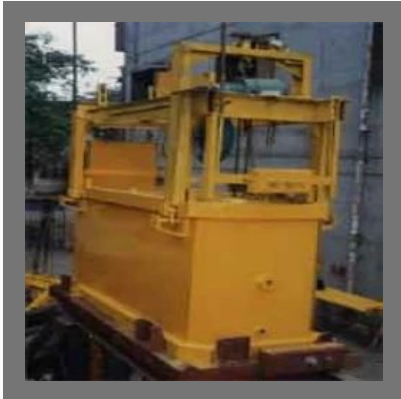
Low Level Radioactive Cell Waste Transportation System
