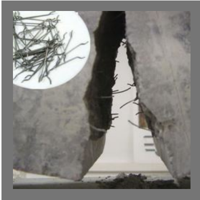
Steel Fibre Concrete
