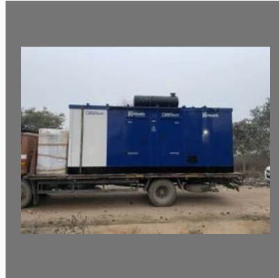
250 Kva Silent Diesel Generator
