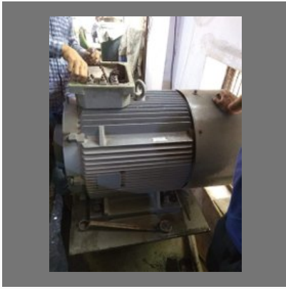
150 Hp Electric Motor, Repairing And Bearing Changing, Along With Servicing
