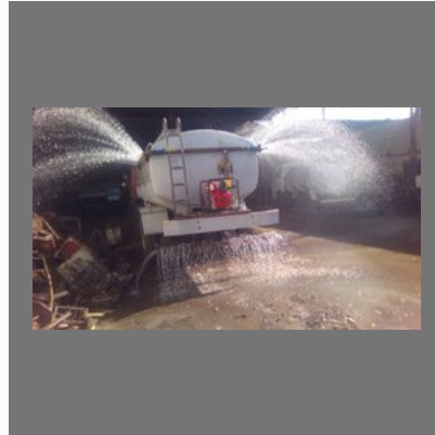
Water Sprinkler Tank
