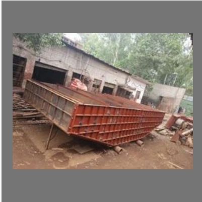
Pier Cap Shutter
