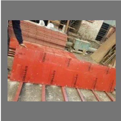
MS Column Shuttering
