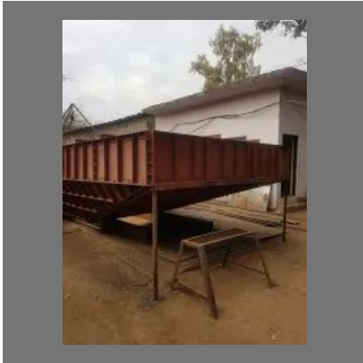
MS Pier Cap Shutter
