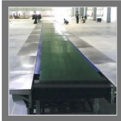
Belt Conveyor with Attached Working Bed
