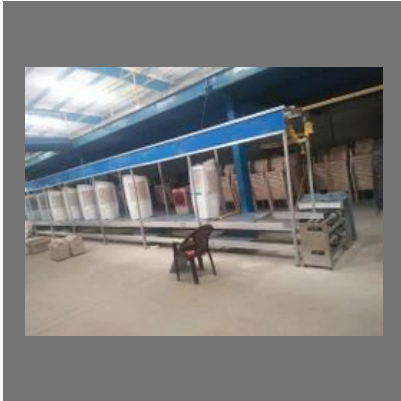
Pallet Transfer Conveyor
