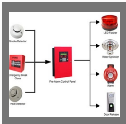
Fire Detection System
