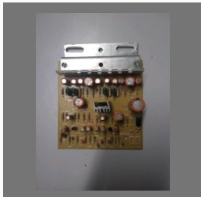
Power Supply Board
