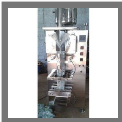
Water Pouch Packing Machine
