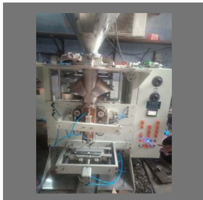
Automatic Powder Packaging Machine
