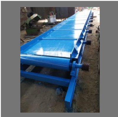
Hot Rolling Mill Conveyor
