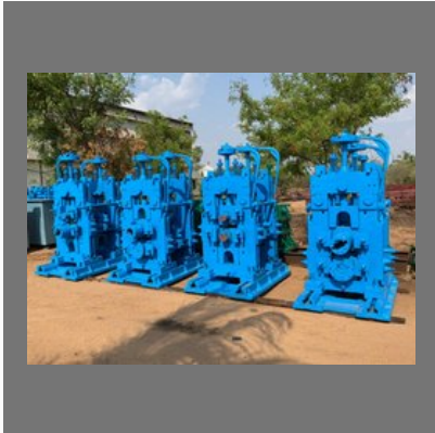
Steel Rolling Mill Stand
