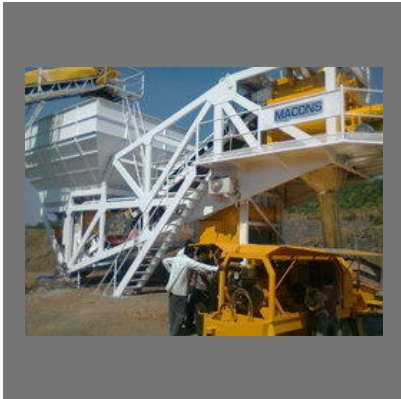
Concrete Batching Plant
