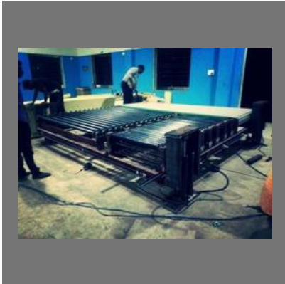
Hydraulic Lifter Conveyors
