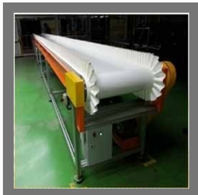
Sidewall Belt Conveyor
