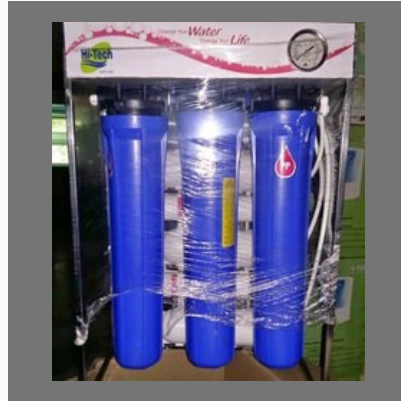
Industrial RO Water Filter
