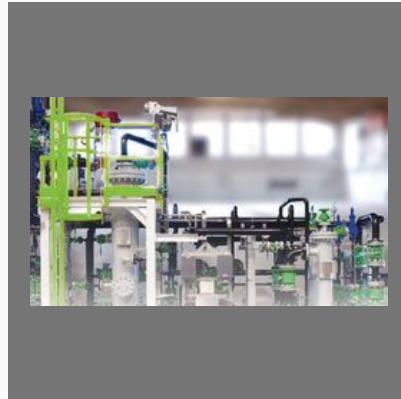
Gas Conditioning Skids
