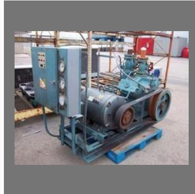
Used Refrigeration Compressor
