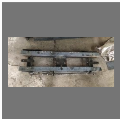
Elevator Guide Rails
