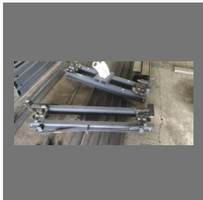
Elevator Guide Rails
