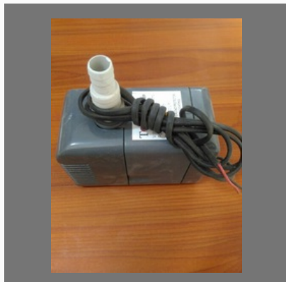
Cooler Water Pump
