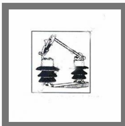
Drop Out Fuse
