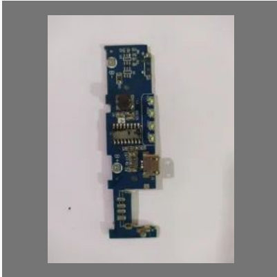
5volt 1amp smps circuit board.
