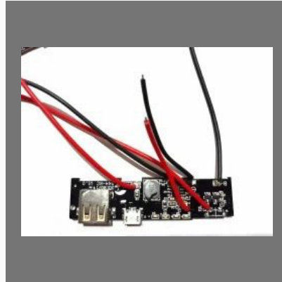
5volt 2amp smps circuit board. With USB
