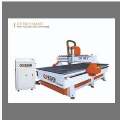
CR-100 V 3 Axis CNC Router Wood Carving Machine
