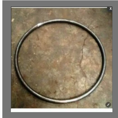
Pipe Dia 33.40 x 3 Thk Make Dia 900mm Through Rolling
