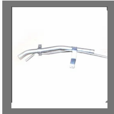
Fuel Tank Filler Pipe
