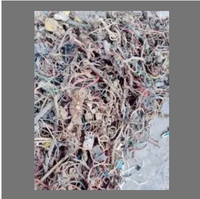
Shredded ICW wire scrap
