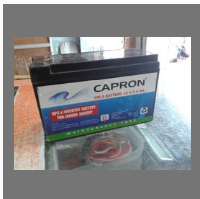
12v UPS VRLA Battery
