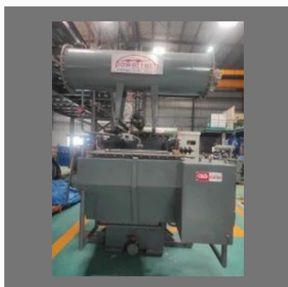
5MVA 33/11KV Power Transformer
