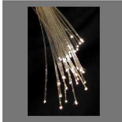
Fiber Optic Cable
