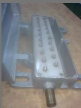
CT Box For Terminating Quad
