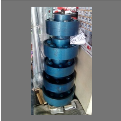
Water Pump Coupling
