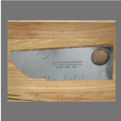
IIW-Type 1 Block 1018 Steel NDT UT Calibration Block
