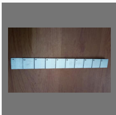
10 Step Block Titanium NDT UTG Calibration Block
