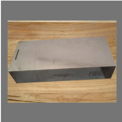
ASME Basic NDT Calibration Block
