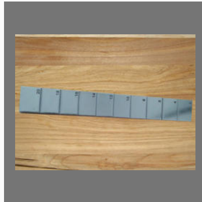
10 Step Block Inconel 600 NDT UTG Calibration Blocks
