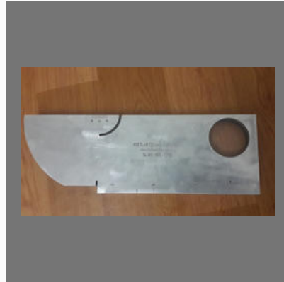
IIW-Type 1 Block 304 Stainless Steel NDT UT Calibration Block
