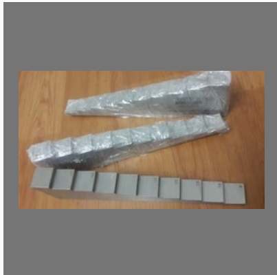
10 Step 90/10 Copper Nickel NDT UTG Calibration Blocks
