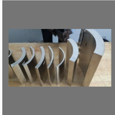
ASME Angle Beam Calibration Block
