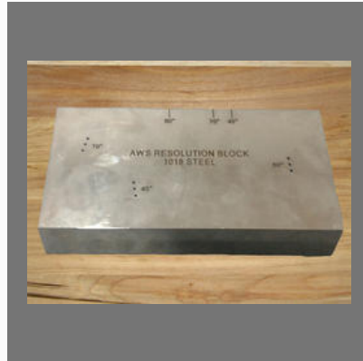
AWS Resolution NDT Calibration Blocks
