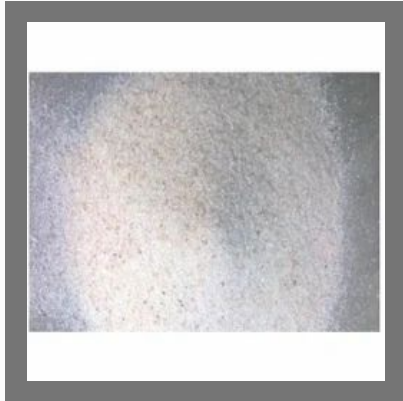
Shot Blasting Quartz Sand
