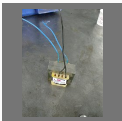
Electric Transformer Coil 230 Input 18 Output
