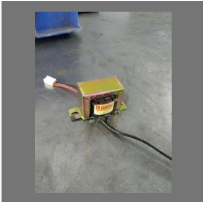
Electric Transformer 230input 909output
