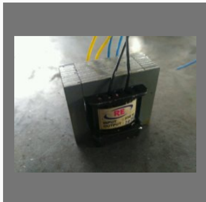
WLG RO Level Censor Transformers
