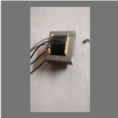
Battery Charger Transformer 6 Volt
