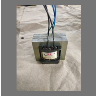
Auto Switch Transformer
