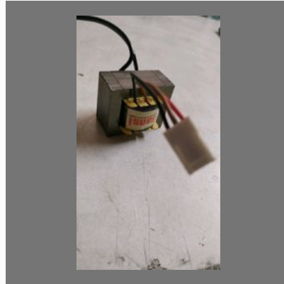
Torchlight Battery Charger Transformer
