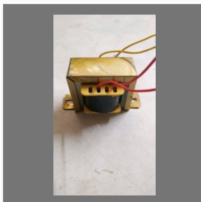
Battery Charger Transformer
