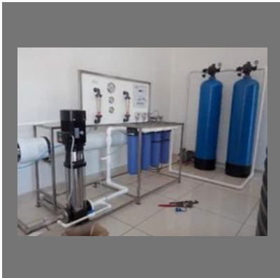
2000 lph R.O Plant
