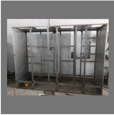
Electrical Control Panel Enclosure
