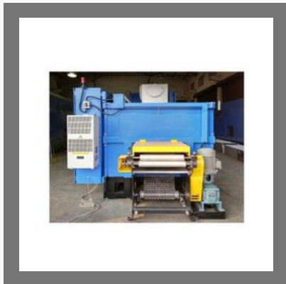
Electrical Conveyor Oven
