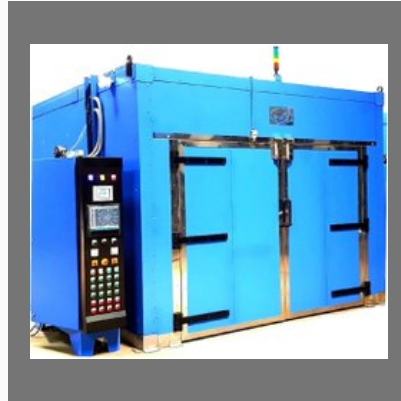
Battery Plate Curing Oven
