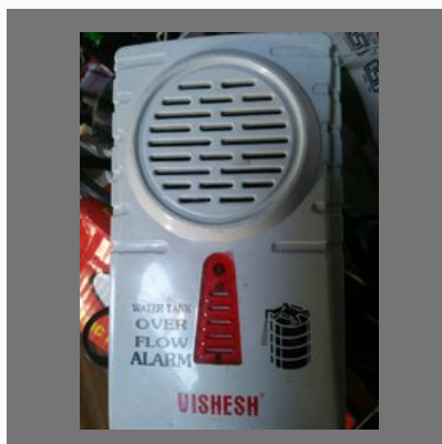
Water Overflow Alarm
