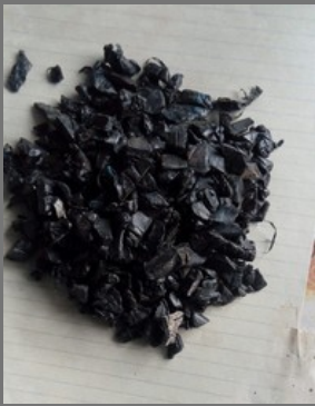
HDPE Pipes Grinding
