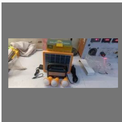
Solar Home Lighting System
