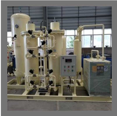
PSA Hospital Oxygen Plant
