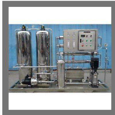
RO Water Plant
