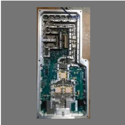
Repair- Comtech BUC 100w
