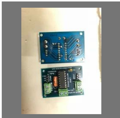
L293d Motor Driver (Robo Inventors)
