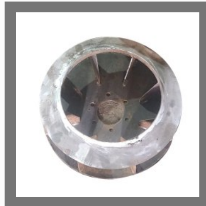
Exhaust Air Blower
